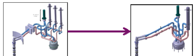
Fig. 5. Evolution of the ASTRID configuration from three SG (125 MWth each) to one single SG (375 MWth).
