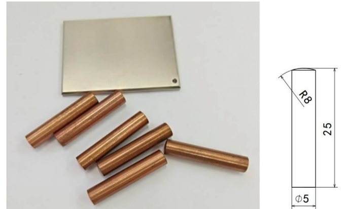
Fig. 8. Configuration of test samples used on HV-MTEST.
