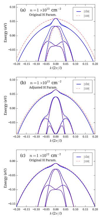
FIG. 6. Valence band structure calculated for  $t_{Si} = 2 \text{ nm}$  (a) with the TB parameters of Ref. 43 for pseudo-hydrogen atoms, (b) with the TB parameters for pseudo-hydrogen atoms adjusted so that the highest valence band is almost isotropic at  $n = 1 \times 10^{13} \text{ cm}^{-2}$ . (c) Same as (a) but at low carrier density  $(n = 1 \times 10^{12} \text{ cm}^{-2})$ . Blue solid lines:  $\mathbf{k} \parallel [1\overline{10}]$ . Red dashed lines:  $\mathbf{k} \parallel [110]$ .
