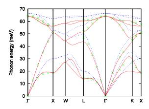
FIG. 13. Phonon band structure of Si calculated using Tersoff<sup>59</sup> (blue dashed lines) and Vanderbilt *et al.*<sup>45</sup> (red solid lines) potentials compared to the experimental data of Ref. 85 (green crosses).
