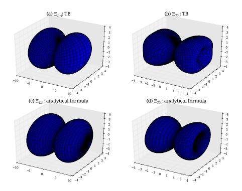
FIG. 11. Angular-dependent deformation potentials for the coupling to LA [(a) and (c)] and TA [(b) and (d)] phonons derived from TB calculations [(a) and (b)], or calculated using Eq. (B2) with  $\Xi_d = 0.91 \text{ eV}$  and  $\Xi_u = 8.70 \text{ eV}$ (c), (d).
