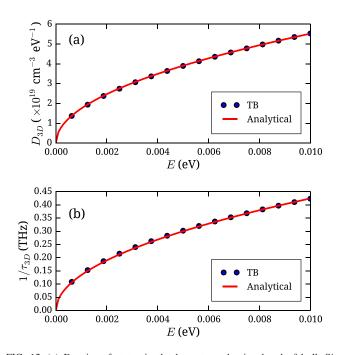
FIG. 12. (a) Density of states in the lowest conduction band of bulk Si (blue dots). The solid line is proportional to  $\sqrt{E}$ . (b) Average scattering rate calculated for electrons on a constant energy surface of the conduction band of bulk Si, versus energy (blue dots). Solid line: analytical fit using Eq. (B3).
