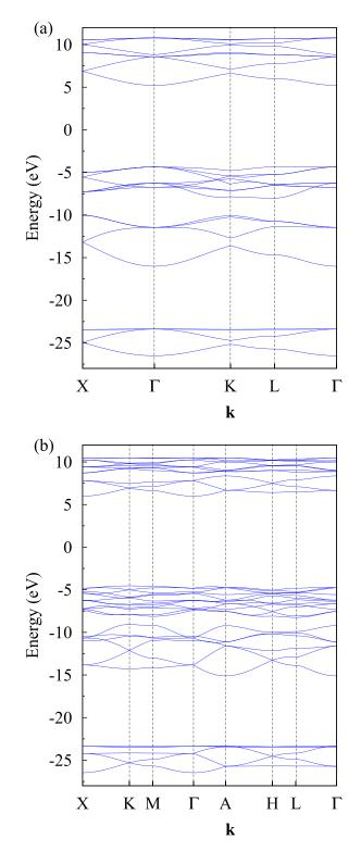
FIG. 14. Band structure of SiO<sub>2</sub> crystals with the  $\beta$ -cristobalite (a) and  $\alpha$ -quartz (b) lattices.
