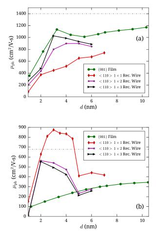
FIG. 8. (a) Phonon-limited electron mobility in (001) Si films with thickness d (green circles), square [110] Si nanowires with side d (red lozenges), and rectangular [110] Si ribbons with sides  $d \times 2d$  (magenta stars) and  $d \times 3d$  (black triangles). The horizontal line indicates the calculated bulk Si mobility. (b) Same for holes.
