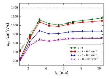
FIG. 2. Phonon-limited electron mobility as a function of the film thickness. Solid lines represent the mobility in the  $[1\bar{1}0]$  direction, dashed lines the mobility in the [110] direction. The horizontal line at 1407 cm<sup>2</sup>/V s indicates the bulk Si mobility.
