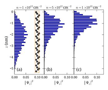
FIG. 3. The unit cell of a Si film ( $t_{Si} = 5$  nm, inset of (a)) and the squared electron wave function of the conduction band minimum at different bias corresponding to (a)  $n = 10^{12}$ , (b)  $n = 5 \times 10^{12}$ , and (c)  $n = 10^{13}$  cm<sup>-2</sup>.
