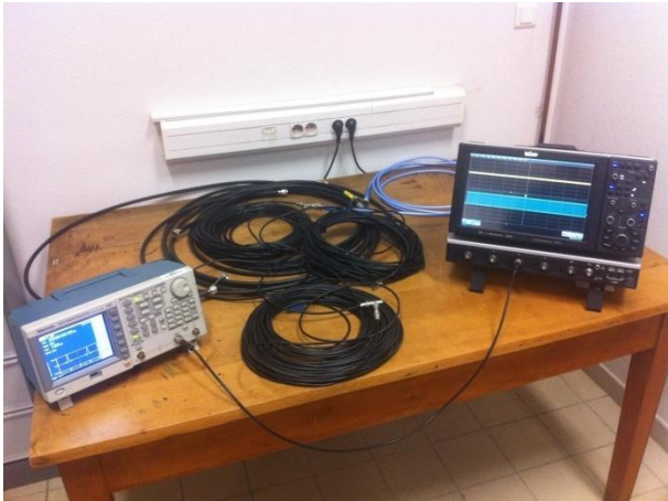
Fig. 8: Picture of the experimental set up. From left to right: the arbitrary waveform generator, the coaxial cable and the numerical oscilloscope.
