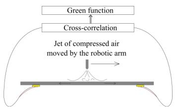
Figure 4 : Process of acquisition for passive tomography
