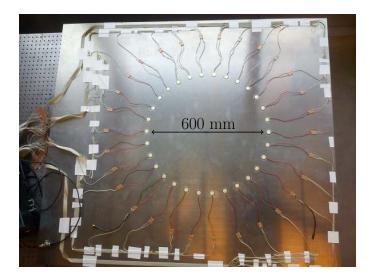
Figure 2 : 30 piezoelectric transducers (Ø 18 mm) glued on the 2 mm thick aluminum plate
