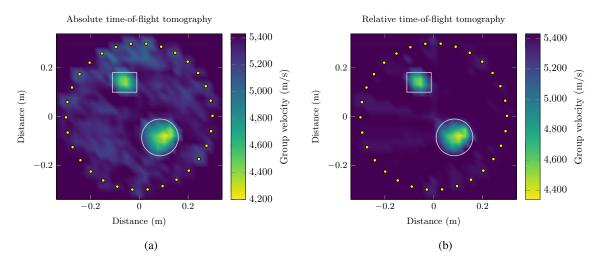
Figure 6 : Active time-of-flight tomography using the Simultaneous Algebraic Reconstruction Technique (SART [6, page 275])
