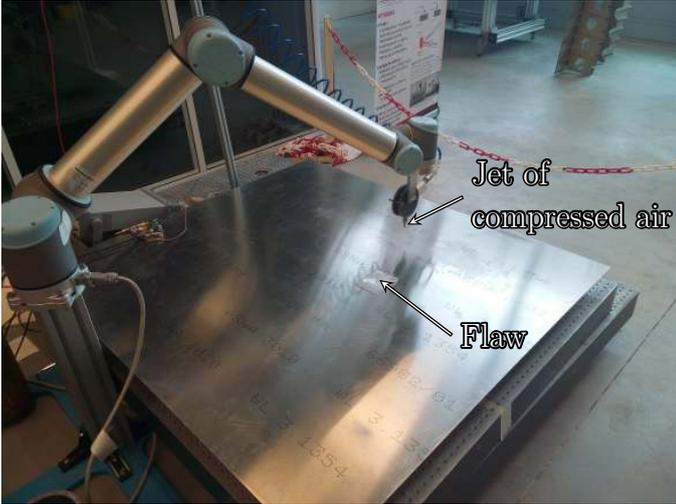
Figure 3 : Experimental setup for passive tomography
