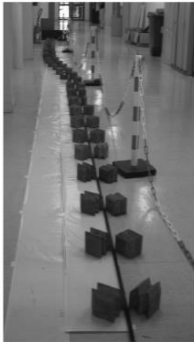
Figure 9. Experimental set-up for '3D' cable bending calibration.
