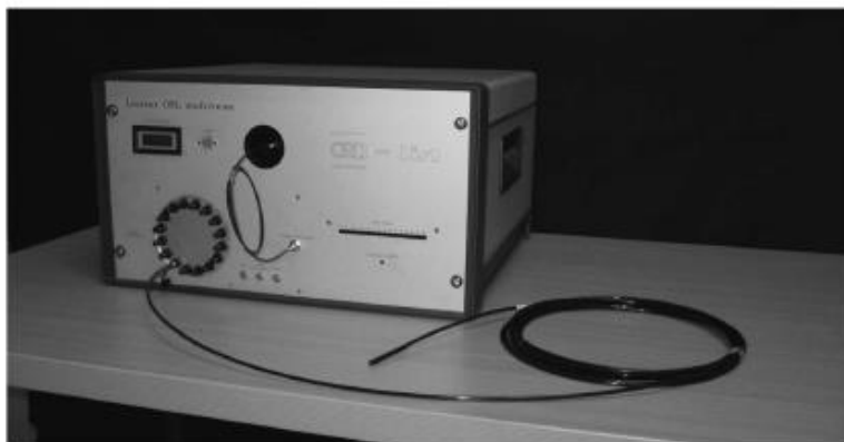
Figure 11. OSL/RL dosimeter developed by the CEA LIST.
