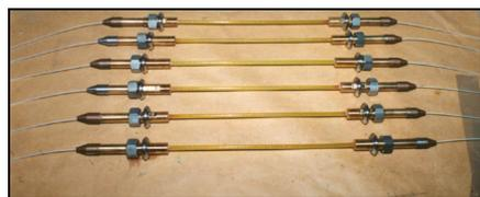
Figure 14. Composite-based FBG extensometers for civil engineering applications. Courtesy of CEA/Magne.
