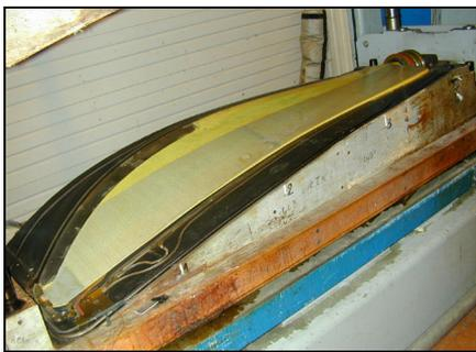
Figure 4. Propeller blade mold, with FBG sensors installed, after curing. Courtesy of Ratier-Figeac, France.
