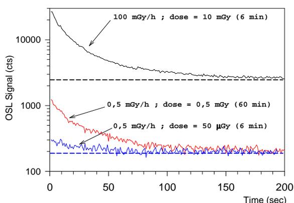
FIG. 6 : Influence of dose and dose-rate on the optical signal
