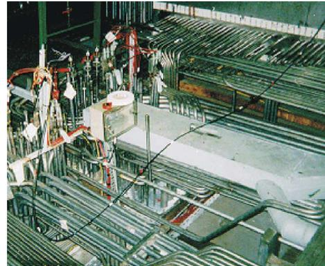
FIG. 8 : Use of the first generation OSL system for remote inspection of small pipes.
