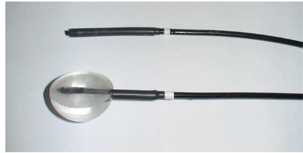
Fig. 1. OSL/FO sensor (top) and mounted with a PMMA build-up cap for surface measurements (bottom).
