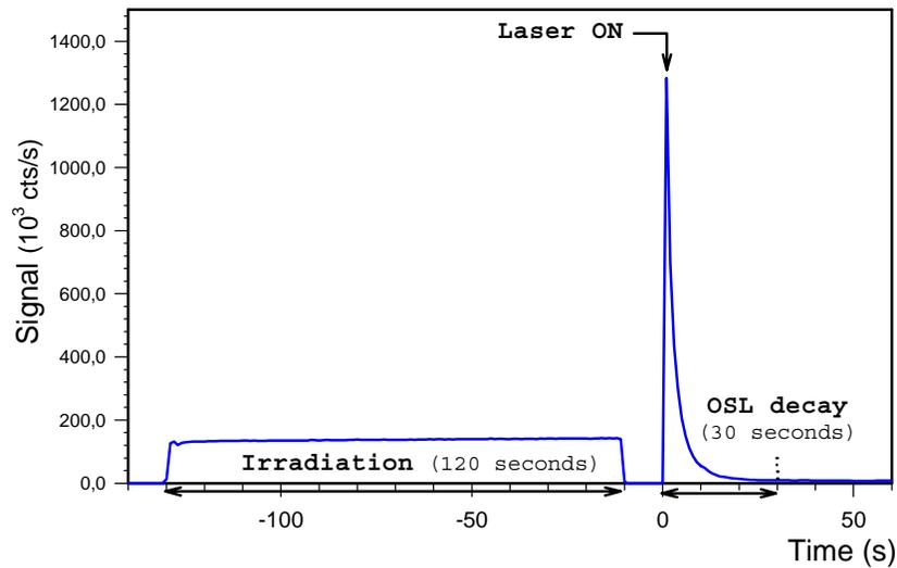
Fig. 2.: Typical RL/OSL signals obtained with the fibre sensors depicted on fig. 1 ( $\dot{D} = 0.15$  Gy/min, Dose = 0.3 Gy)
