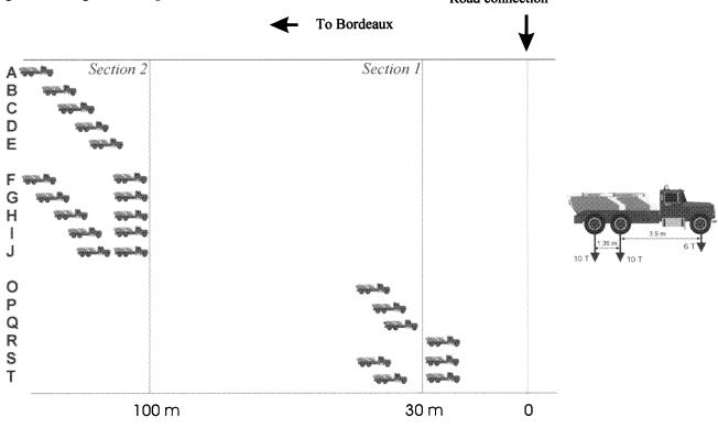
Fig. 10 : Truck movements and associated labels A to J and O to T (each figure symbolizes a series of 4 trucks similar to that described above)
