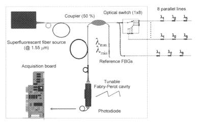
Fig. 1: Acquisition unit for FBG sensing purposes F built in an industrial PC
