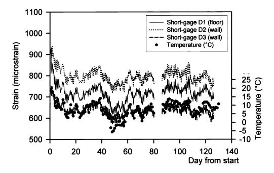
Fig. 15: Strain and temperature data gathered during field test on line D
