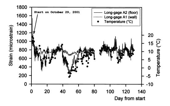
Fig. 12 : Strain and temperature data gathered during field test on line A
