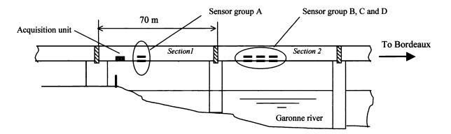
Fig. 6 : Access to the bridge and installation of the optical instrumentation
