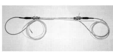
Fig. 3: Short-Gage Extensometer (SGE) (FBG bonded on steel)
