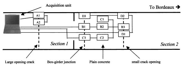
Fig. 7: Installation scheme of the extensioneters inside the central tunnel of the Saint-Jean bridge (seen from top)
