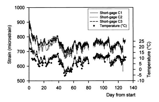
Fig. 14 : Strain and temperature data gathered during field test on line C (all extensometers are fixed onto the floor)
