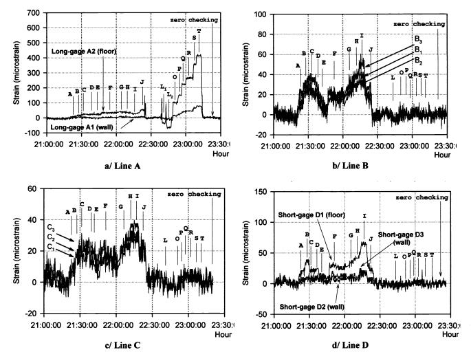
Fig. 11 : Loading-induced strain during the standardized loading test (corrected from thermo-mechanical influence) observed for each line. a/ line A (FBG-LGE); b/ line B (FBG-LGE), c/ line C (FBG-SGE), d/ line D (FBG-SGE)
