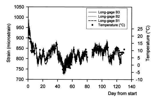
Fig. 13: Strain and temperature data gathered during field test on line B (all extensometers are fixed onto the floor)
