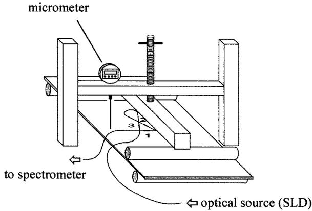
Fig. 2. Four-point bending setup: SLD, superluminescent diode.
