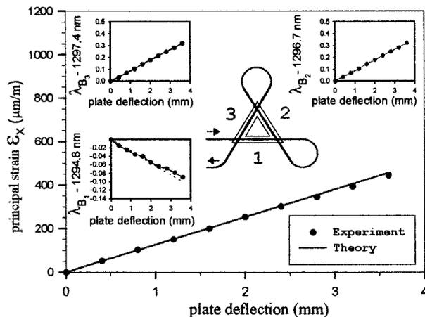
Fig. 4. Experimental and theoretical evolutions of the Bragg grating wavelengths under an increased load for  $0^\circ$  orientation (FBG 1 is aligned along the Y principal axis) and experimental and theoretical evaluations of the principal strain  $\epsilon_X$ .
