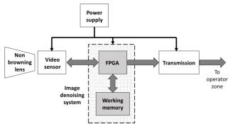
Fig. 1. Architecture of the hardened camera including the image denoising system.
