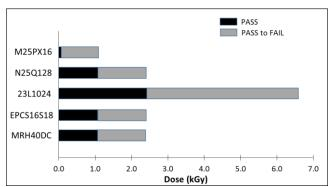
Fig. 5. TID response of the memory devices tested in this work.
