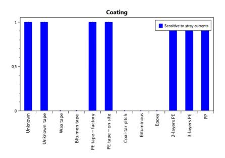
Figure 3: Coating types that are sensitive to stray currents
