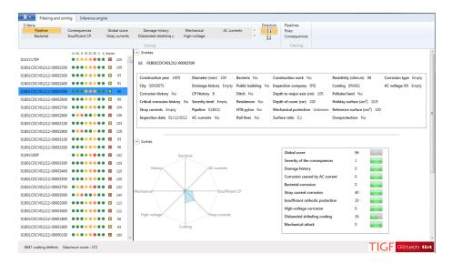
Figure 5: Dedicated user interface with a synthetic view of all the DCVG defects (left part), and a detailed view of a particular defect with its parameter values and the inferred corrosion risks (right part).
