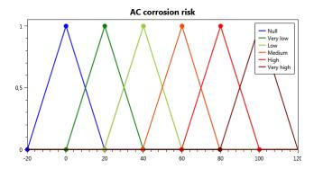
Figure 2: Fuzzy sets for risk level, in this case for alternating current corrosion
