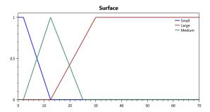
Figure 4: Fuzzy sets defined for the estimated defect surface
