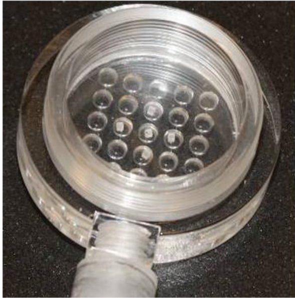
Figure 1. PMMA holder designed to position cubic TLDs of 1 mm side length vertically during photon exposures in air. This configuration shows five dosimeters located in the central TLD wells.
