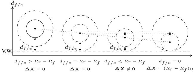
Fig. 4. Positions of the avatars of the finger and ring in function of the distance to the virtual wall. Dashed circles: ring; plain circles: finger; single-headed arrows:  $\Delta X$ . V.W.: virtual wall.
