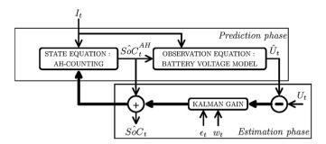
**Fig. 3.** SoC estimator through an extended Kalman filter, where  $I_t$  is the input  $u_t$ . SoC<sub>t</sub> the state variable  $x_t$  and  $U_t$  the observed variable  $y_t$ .
