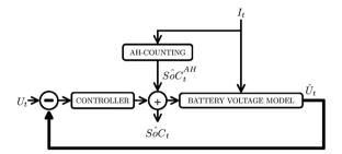
Fig. 2. Concept of SoC adjustment through a controller.
