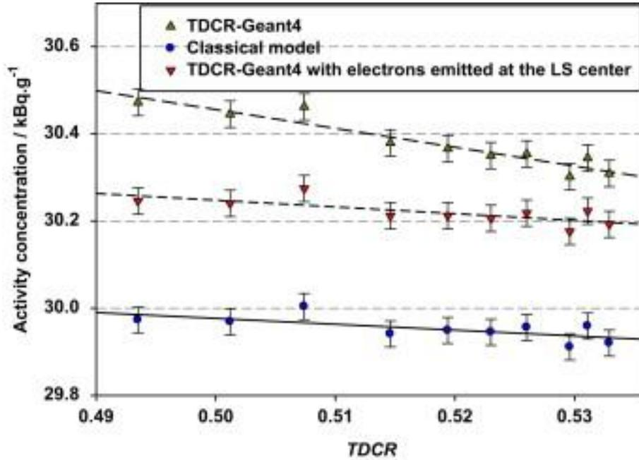
Fig. 7. Activity concentration versus  $TDCR$  value in the case of  ${}^3\text{H}$  in UG obtained with both statistical and TDCR-Geant4 models ( $kB$  equal to  $0.13 \text{ mm MeV}^{-1}$ ).
