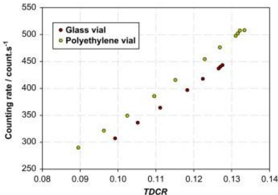
Fig. 3. Comparison between polyethylene and glass vials of double-coincidence counting rates versus *TDCR* values for x-ray photons of 2.7 keV (the collimator was not used).
