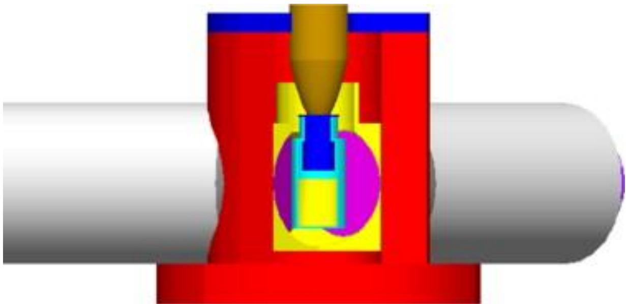
Fig. 1. Geometrical modeling with Geant4 of the LS-counter vial coupled with the miniature x-ray tube. The collimator (used for  $[kB; S]$  measurements) is also included inside the vial, which was hung between PMTs in the optical cavity.
