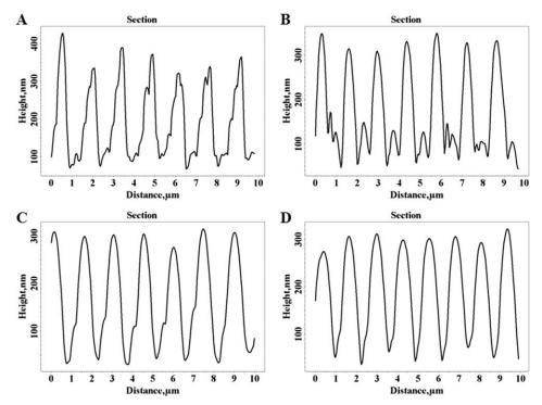
Figure 6. AFM images (cross sections) of the SRGs corresponding to sample 3 obtained with 200 pulses and different fluence values: (A) 4.3, (B) 8.8, (C) 14.2, and (D) 16.5 mJ/cm<sup>2</sup>. The film thickness was 500 nm, and the SRG periodicity was 1.4  $\mu$ m.
