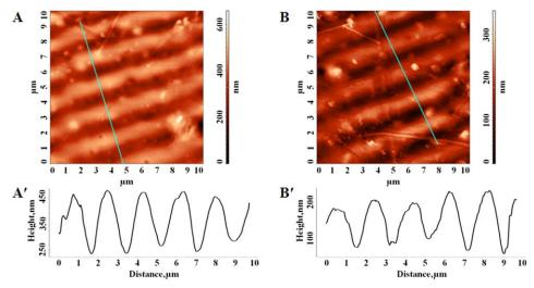
Figure 10. AFM images of the SRGs corresponding to sample 5: (A) laser fluence of 28.3 mJ/cm and 20 pulses and (B) laser fluence of 28.3 mJ/cm<sup>2</sup> and 50 pulses. The film thickness was 600 nm, and the SRG periodicity was 2  $\mu$ m. [Color figure can be viewed in the online issue, which is available at wileyonlinelibrary.com.]
