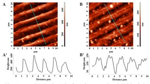
**Figure 7.** AFM images of the SRGs corresponding to sample 4: (A) laser fluence of 24.5 mJ/cm and 30 pulses (relief amplitude = 400 nm) and (B) laser fluence of 17.4 mJ/cm and 80 pulses (relief amplitude = 200 nm). The film thickness was 500 nm, and the SRG periodicity was 2  $\mu$ m. [Color figure can be viewed in the online issue, which is available at wileyonlinelibrary.com.]
