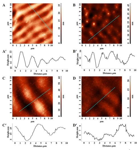
**Figure 2.** AFM images of the SRGs corresponding to sample 2 registered 14 days after inscription: (A) fluence of 14 mJ/cm<sup>2</sup> and 100 pulses, (B) fluence of 8.8 mJ/cm<sup>2</sup> and 100 pulses, (C) fluence of 13.8 mJ/cm<sup>2</sup> and 100 pulses, and (D) fluence of 11.8 mJ/cm<sup>2</sup> and 100 pulses. The film thicknesses were (A,B) 500 and (C,D) 1000 nm. [Color figure can be viewed in the online issue, which is available at wileyonlinelibrary.com.]
