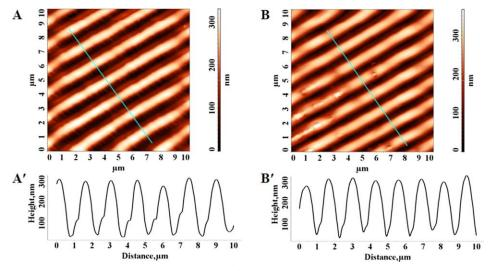
**Figure 4.** AFM images of the SRG corresponding to sample 3: (A) laser fluence of 14 mJ/cm and 200 pulses (relief amplitude = 300 nm) and (B) laser fluence of 16.5 mJ/cm and 200 pulses (relief amplitude = 300 nm). The film thickness was 500 nm, and the SRG periodicity was 1.4  $\mu$ m. [Color figure can be viewed in the online issue, which is available at wileyonlinelibrary.com.]
