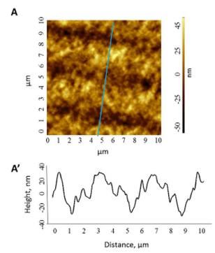
**Figure 11.** AFM image of the CF<sub>3</sub>–Azo–Psi film irradiated with a 488-nm laser wavelength (relief amplitude = 55 nm, SRG periodicity = 4.3  $\mu$ m, film thickness = 740 nm). [Color figure can be viewed in the online issue, which is available at wileyonlinelibrary.com.]
