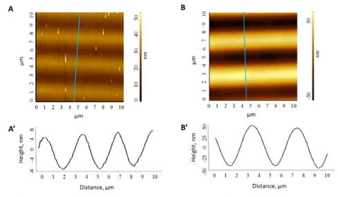
**Figure 3.** AFM images of the Azo–Psi film irradiated with (A) a 350-nm laser wavelength (relief amplitude = 12 nm, SRG periodicity = 2.8  $\mu$ m) and (B) a 488-nm laser wavelength (relief amplitude = 96 nm, SRG periodicity = 4  $\mu$ m). [Color figure can be viewed in the online issue, which is available at wileyonlinelibrary.com.]
