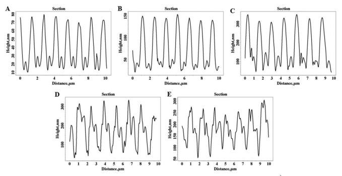
Figure 5. AFM images (cross sections) of the SRGs corresponding to sample 3 obtained with a fluence value of 8.8 mJ/cm<sup>2</sup> and different numbers of pulses: (A) 50, (B) 100, (C) 200, (D) 300, and (E) 500. The film thickness was 500 nm, and the SRG periodicity was 1.4  $\mu$ m.
