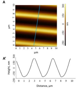
**Figure 8.** AFM image of the SRGs corresponding to sample 4 with a laser fluence of 15.5 mJ/cm and 180 pulses (relief amplitude = 405 nm). The film thickness was 500 nm, and the SRG periodicity was 2  $\mu$ m. [Color figure can be viewed in the online issue, which is available at wileyonlinelibrary.com.]
