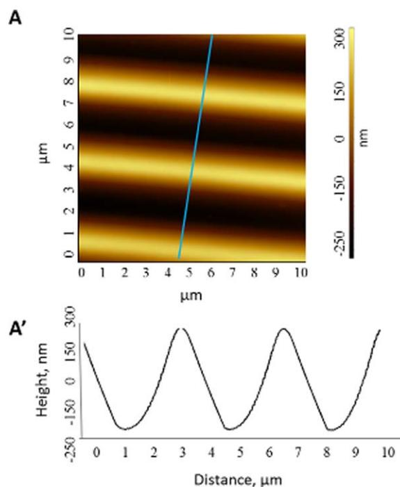
**Figure 9.** AFM image of the Naph-Azo-Psi film irradiated with a 488-nm laser wavelength (relief amplitude = 530 nm, SRG periodicity = 3.6  $\mu\text{m}$ , film thickness = 700 nm). [Color figure can be viewed in the online issue, which is available at [wileyonlinelibrary.com](http://wileyonlinelibrary.com).]
