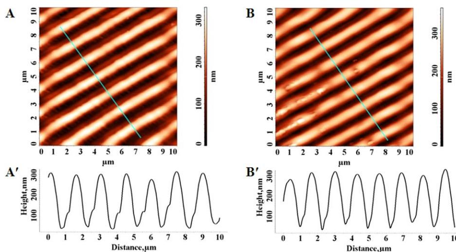
**Figure 4.** AFM images of the SRG corresponding to sample 3: (A) laser fluence of  $14 \text{ mJ/cm}^2$  and 200 pulses (relief amplitude = 300 nm) and (B) laser fluence of  $16.5 \text{ mJ/cm}^2$  and 200 pulses (relief amplitude = 300 nm). The film thickness was 500 nm, and the SRG periodicity was  $1.4 \mu\text{m}$ . [Color figure can be viewed in the online issue, which is available at [wileyonlinelibrary.com](http://wileyonlinelibrary.com).]
