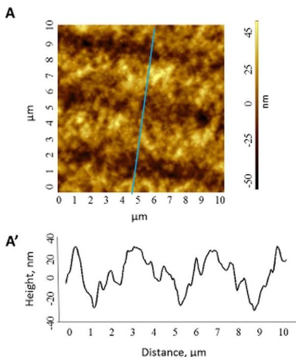
**Figure 11.** AFM image of the CF<sub>3</sub>–Azo–Psi film irradiated with a 488-nm laser wavelength (relief amplitude = 55 nm, SRG periodicity = 4.3 μm, film thickness = 740 nm). [Color figure can be viewed in the online issue, which is available at [wileyonlinelibrary.com](http://wileyonlinelibrary.com).]
