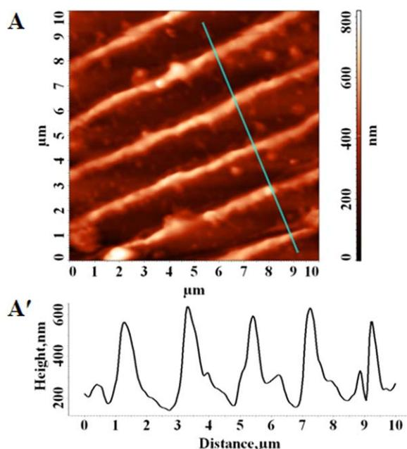
**Figure 8.** AFM image of the SRGs corresponding to sample 4 with a laser fluence of 15.5 mJ/cm and 180 pulses (relief amplitude = 405 nm). The film thickness was 500 nm, and the SRG periodicity was 2  $\mu\text{m}$ . [Color figure can be viewed in the online issue, which is available at [wileyonlinelibrary.com](http://wileyonlinelibrary.com).]
