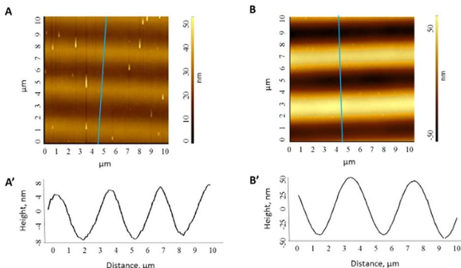
**Figure 3.** AFM images of the Azo-Psi film irradiated with (A) a 350-nm laser wavelength (relief amplitude = 12 nm, SRG periodicity =  $2.8 \mu\text{m}$ ) and (B) a 488-nm laser wavelength (relief amplitude = 96 nm, SRG periodicity =  $4 \mu\text{m}$ ). [Color figure can be viewed in the online issue, which is available at [wileyonlinelibrary.com](http://wileyonlinelibrary.com).]
