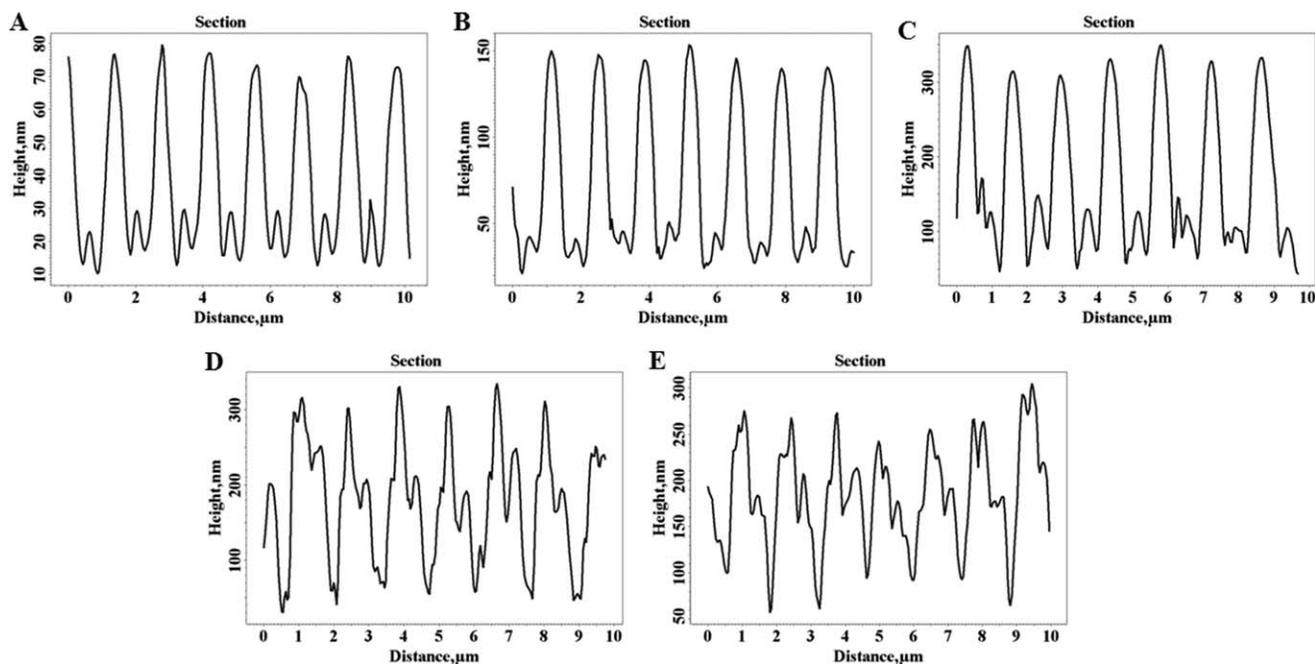
**Figure 5.** AFM images (cross sections) of the SRGs corresponding to sample 3 obtained with a fluence value of  $8.8 \text{ mJ/cm}^2$  and different numbers of pulses: (A) 50, (B) 100, (C) 200, (D) 300, and (E) 500. The film thickness was 500 nm, and the SRG periodicity was  $1.4 \mu\text{m}$ .
