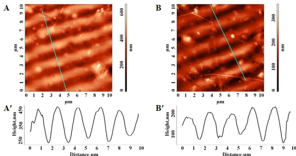
**Figure 10.** AFM images of the SRGs corresponding to sample 5: (A) laser fluence of 28.3 mJ/cm<sup>2</sup> and 20 pulses and (B) laser fluence of 28.3 mJ/cm<sup>2</sup> and 50 pulses. The film thickness was 600 nm, and the SRG periodicity was 2 μm. [Color figure can be viewed in the online issue, which is available at [wileyonlinelibrary.com](http://wileyonlinelibrary.com).]
