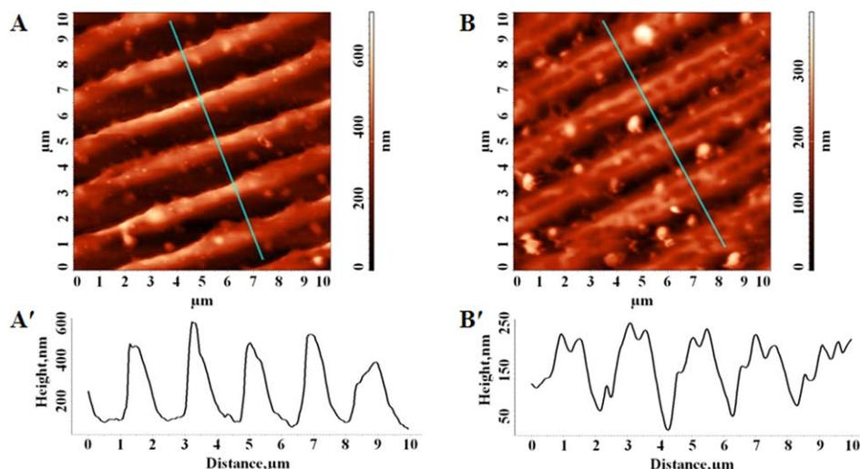
**Figure 7.** AFM images of the SRGs corresponding to sample 4: (A) laser fluence of 24.5 mJ/cm and 30 pulses (relief amplitude = 400 nm) and (B) laser fluence of 17.4 mJ/cm and 80 pulses (relief amplitude = 200 nm). The film thickness was 500 nm, and the SRG periodicity was 2  $\mu\text{m}$ . [Color figure can be viewed in the online issue, which is available at [wileyonlinelibrary.com](http://wileyonlinelibrary.com).]
