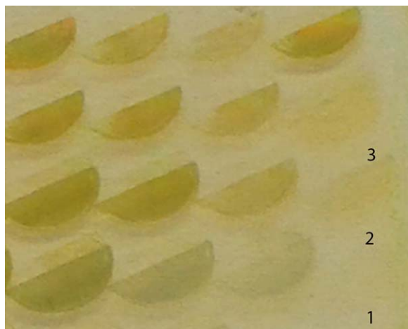
Figure 1. Picture of the different SRG regions (corresponding to sample 1) generated on the film surface. The relief instability can be observed from the disappearance of SRGs (points 1–3). [Color figure can be viewed in the online issue, which is available at wileyonlinelibrary.com .]
