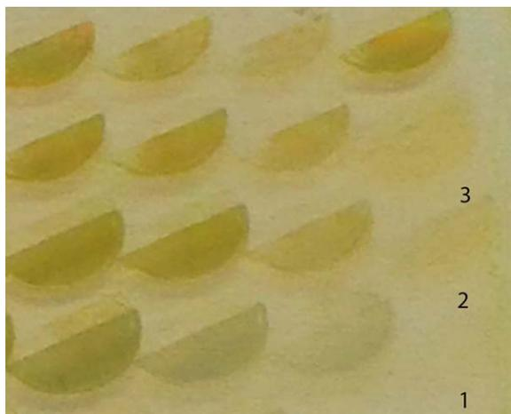
**Figure 1.** Picture of the different SRG regions (corresponding to sample 1) generated on the film surface. The relief instability can be observed from the disappearance of SRGs (points 1–3). [Color figure can be viewed in the online issue, which is available at [wileyonlinelibrary.com](http://wileyonlinelibrary.com).]
