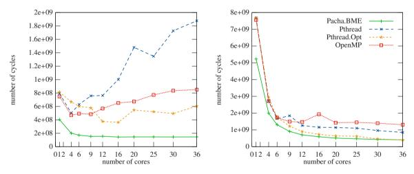
Fig. 4. Executing time of the pedestrian detection application running on a TILEPro64 with PACHA+BME or using Linux with common parallel programming libraries (a) Pre-processing (b) Classification
