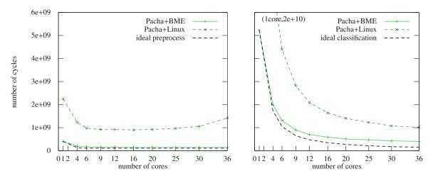
Fig. 2. Evaluation of the Linux back-end and the close-to-hardware back-end on TILEPro64. Execution time for (a) the pre-processing part (b) the classification part
