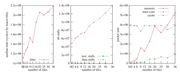
Fig. 3. Profiling macro-blocs of the classification, (a) the execution time median for a macro-bloc, (b) the instructions stalls and data stalls, (c) the network profiling, number of packets sent through cache coherency network, inter-core network and memory network
