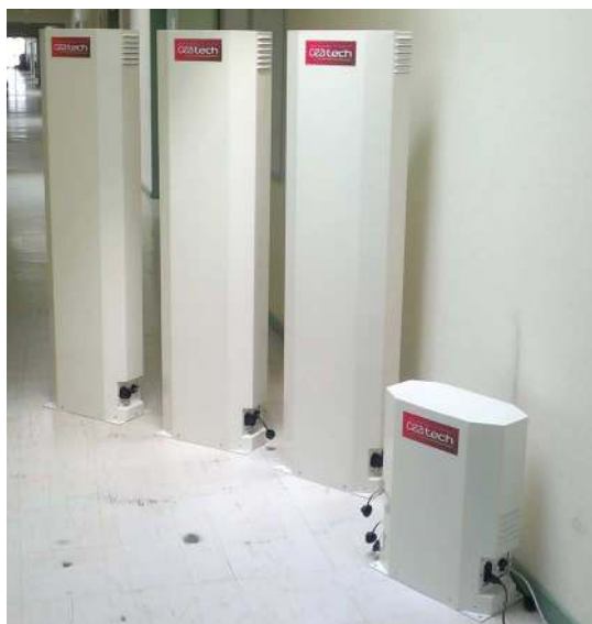
Fig. 11. RPMs network prototype showing three long detection units and a small control unit.
