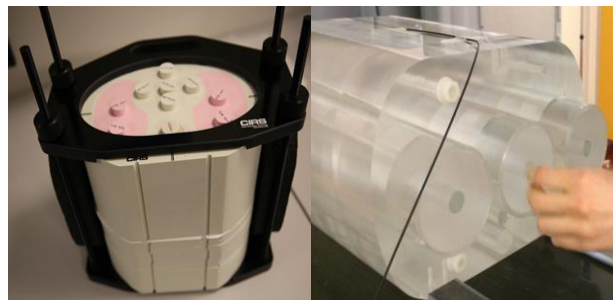
Figure 7: CIRS (left) and DTU phantoms.
