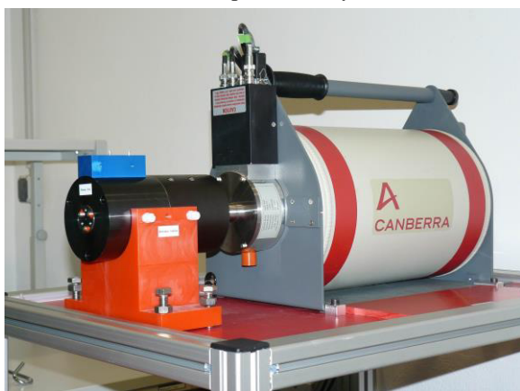
Figure 4: PTB Ge spectrometer assembly
