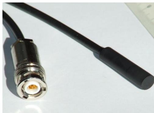
Figure 5: prototype of the Tor vergata/ENEA diamond based dosimeter.
