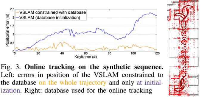
Fig. 3. Online tracking on the synthetic sequence. Left: errors in position of the VSLAM constrained to the database on the whole trajectory and only at initialization. Right: database used for the online tracking
