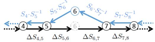
Fig. 1. Illustration of the third step of the database construction. In this example the 6<sup>th</sup> key-frame has an absolute pose associated and is shifted towards it, resulting in large errors  $r_{5,6}$  and  $r_{6,7}$  (see equation (3)) that are minimized through pose-graph optimization while fixing the 6<sup>th</sup> camera pose.
