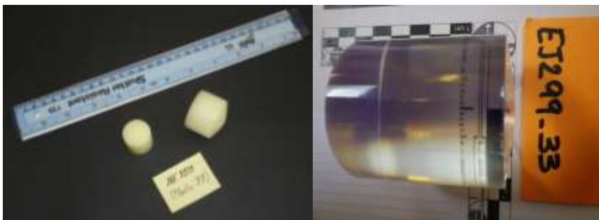
Figure 32. Pictures of NE-150 (left) and EJ-299-33 (right) after whitening and/or dishing of the morphology (Copyright F. Brooks for left picture, Copyright CEA for right picture).
