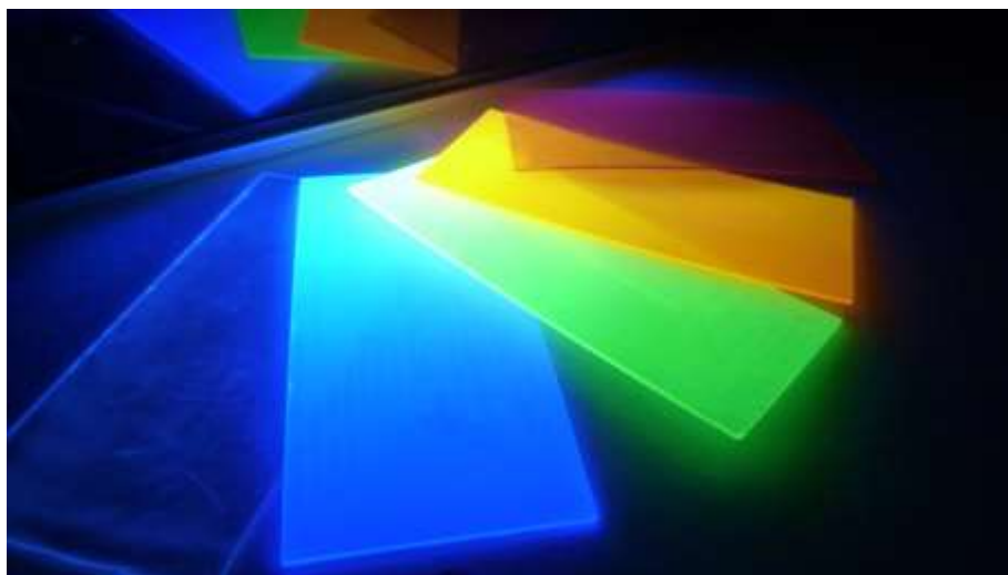
Figure 1. Plastic scintillators displaying different emission wavelengths (excitation with UV lamp; copyright CEA).
