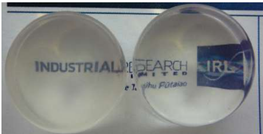
Figure 7. Photo of scintillator samples, 1.25 wt% enriched LiMA (left) and 10 wt% enriched LiMA (right). Diameters are 20 mm, thicknesses 10 mm (reproduced with permission from ref 35. Copyright 2013 Elsevier B. V.).
