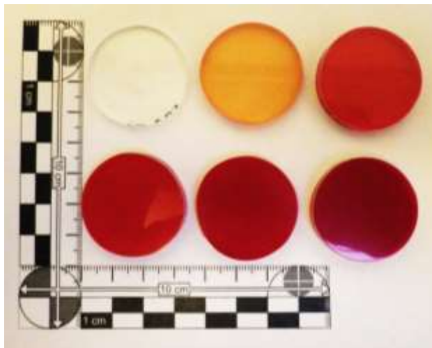
Figure 29. Cross-linked scintillators with increasing loading of Ir(piq) 2 (acac) (0 – 0.1 wt%).
