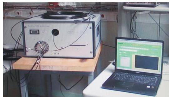
Fig. 5 OSL Instrument: 16 channels ; Range 100 m (Transducers  $\text{Al}_2\text{O}_3$  – Visible spectrum Range.
