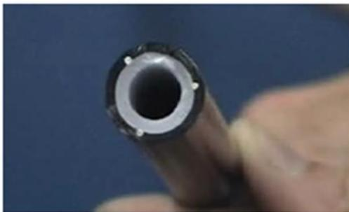
Fig. 4 Multi-parameters cable to simultaneously determine: strain, curvature, plane of curvature and temperature profiles.
