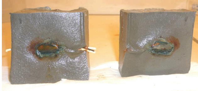
Figure 4 – Fracture of the cement paste sample due to internal strains caused by accumulation of corrosion products
