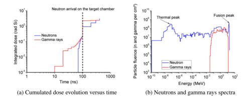
Figure 1. Simulation of radiative environment at 4 m from TCC for a neutron yield of 10<sup>16</sup>.
