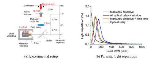
Figure 4. Behaviour of the catadioptric relay under irradiation on ELSA facility.
