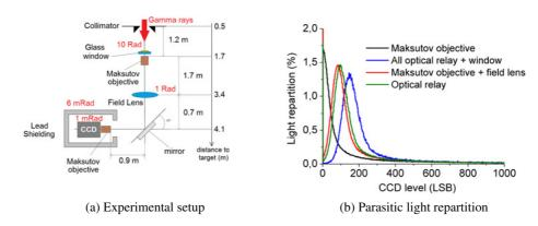
Figure 4. Behaviour of the catadioptric relay under irradiation on ELSA facility.
