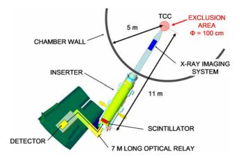
Figure 2. Diagnostic implantation in the LMJ facility.
