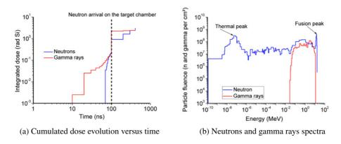
Figure 1. Simulation of radiative environment at 4 m from TCC for a neutron yield of 10<sup>16</sup>.
