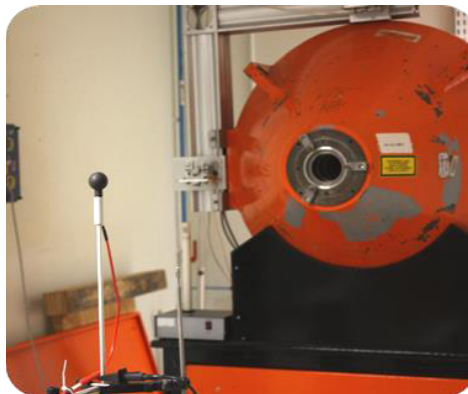
Figure 6. Ionization chamber in the ^{60}\text{Co} beam of LNE-LNHB
