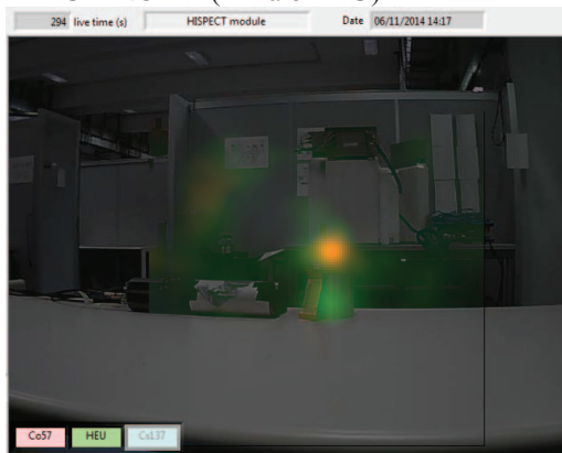
Figure 5: Example of a 5 min image acquired by Hispect camera with a 55g HEU sample (automatically identified by the software in green) at 1 meter and a masking ^{57}\text{Co} source (16.8 MBq, identified in red).
