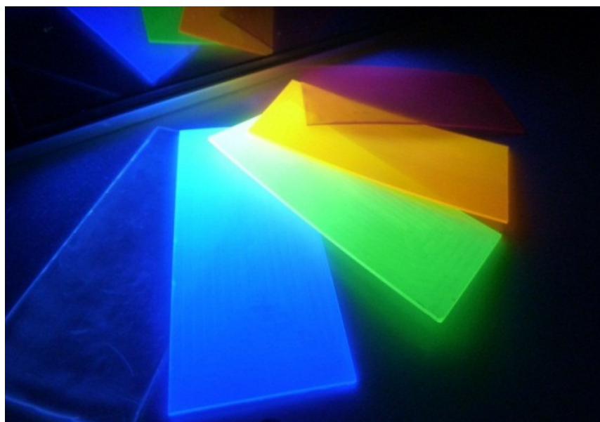
Figure 1. Plastic scintillators displaying different emission wavelengths (excitation with UV lamp; © CEA).
