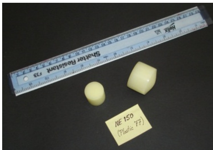
Figure 10: Picture of a degraded NE-150 plastic scintillator (© F.D. Brooks, with permission).
