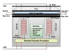
Fig. 5. Internal view of an FU comprising two dual-clocked FIFOs.
