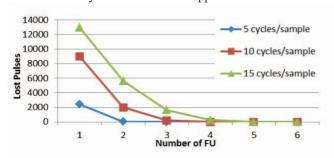
Fig. 6. Simulation results for one acquisition channel compared to the number of FUs required to reach the zero dead-time.
