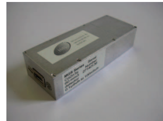
Figure 1: IMS miniature embedded CdZnTe crystal gamma-ray spectrometer
