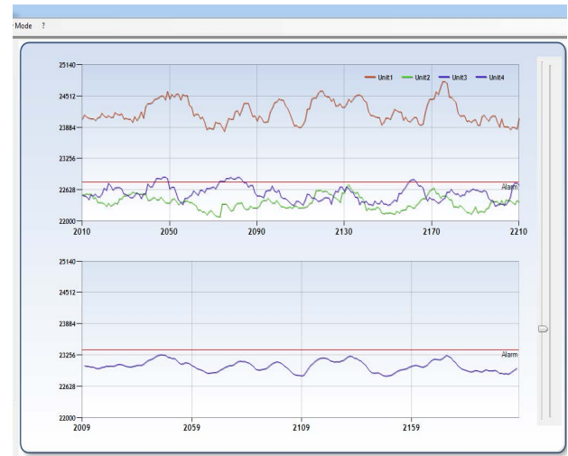
Fig 8. ^{137}\text{Cs} source static close to channel 1 with ^{60}\text{Co} as background source (after delay adjustment)
