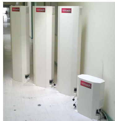
Fig 3. Prototype system with 3 sensor units and a control command unit
