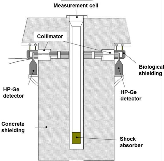
Fig. 1: Schematic view for the burn-up measurement cell, called station 1
