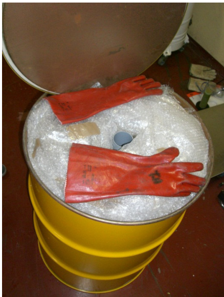
Fig. 6. Mock-up drum containing a 0.02\text{ g/cm}^3 vinyl matrix.
