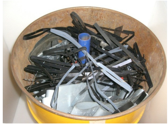
Fig. 7. Mock-up drum containing a 0.22\text{ g/cm}^3 iron matrix.
