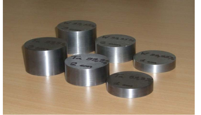
Fig. 12. Tungsten and tantalum targets of different thicknesses.
