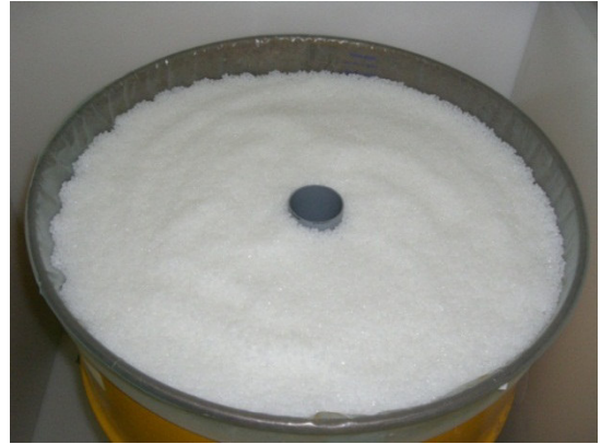
Fig. 8. Mock-up drum containing a 0.45\text{ g/cm}^3 polyethylene matrix.
