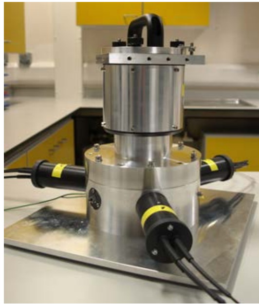
Fig. 4. Optical chamber of the NPL TDCR counter
