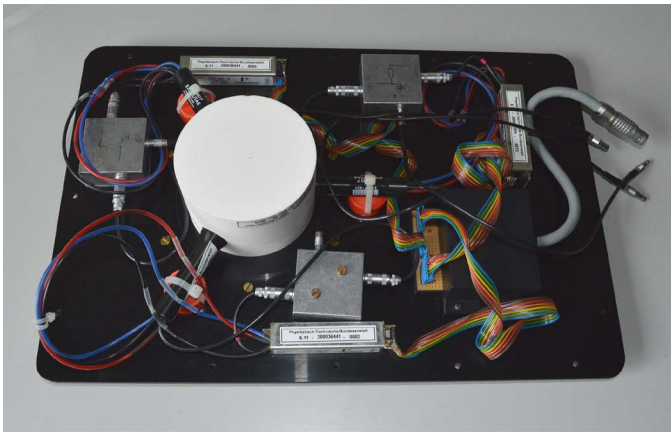
Fig. 6. The PTB TDCR counter with optical chamber, PM tubes and HV supplies.
