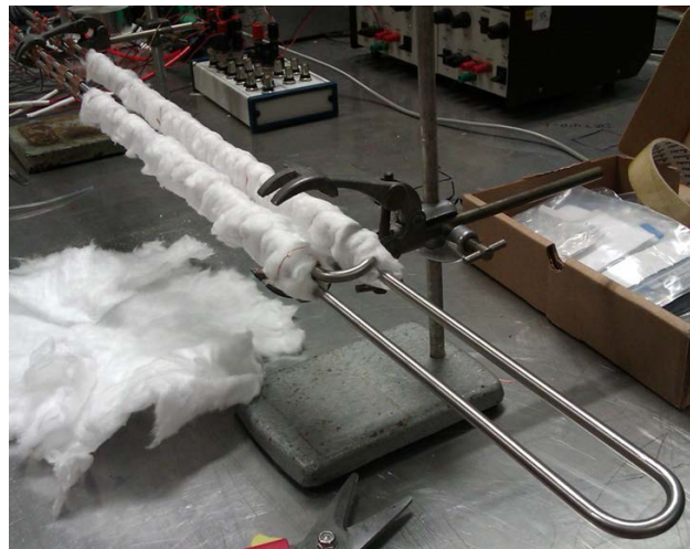
Fig 2. A PAT thermometer made from Inconel. The exposed length of Inconel is the temperature sensitive region.
