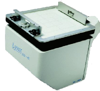
Fig. 4. The FIMEL EPID used for high-energy experiments carried out in the SAPHIR facility.
