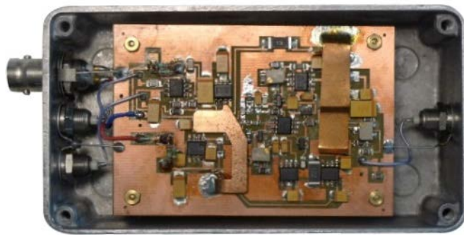
Fig. 1. Example of a dedicated front-end electronic module adapted for use with NaI(Tl) photon detector systems.
