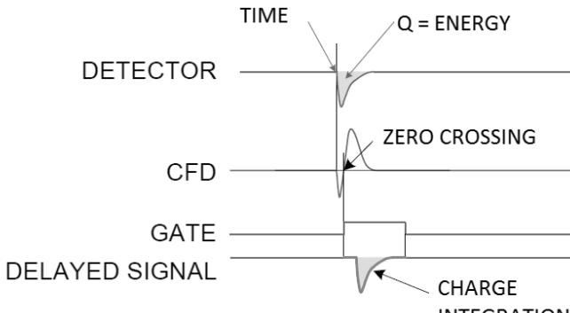
Fig. 7. Digital signals created in the DPP-CI firmware. (Adapted from [9]).
