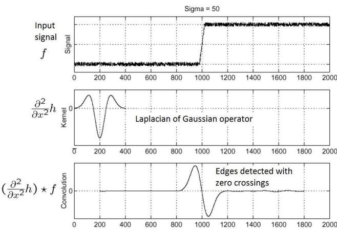
Fig. 3. Recursive Gaussian DPP Filter used for edge detection and timing optimization. The digitized input signal from the front end electronics ( $f$ ) undergoes a convolution with the second derivative (or Laplacian operator) of the Gaussian filter ( $h$ ).
