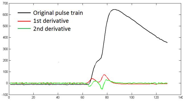
Fig. 4. (x-axis scale: x 64 ns). Example of the use of the algorithm for pile-up identification based on zero-crossing detection using the 2<sup>nd</sup> derivative of the Gaussian filter. The separation between output pulses is  $\sim 600$  ns, which is of the order of the rise time of the input pulse.
