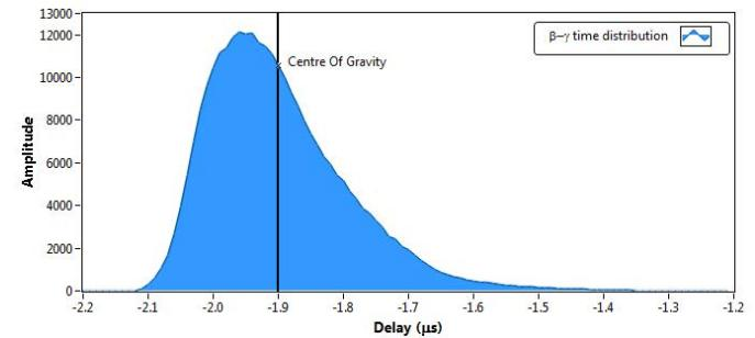
Fig. 11. The time-delay distribution between beta and gamma pulses for a  $^{60}\text{Co}$  source measured in a  $4\pi\beta-\gamma$  configuration at ENEA. The beta channel used was an atmospheric proportional counter and the gamma channel comprised an NaI(Tl) detector. The digitizer used was a CAEN DT5720.
