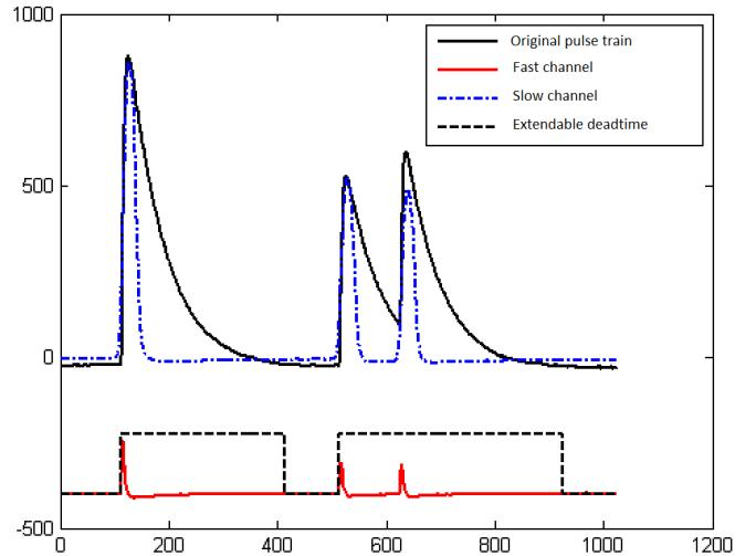
Fig. 5. (x-axis scale: x 64 ns). Digital pulse processing applied to signals delivered by a high-efficiency well-type NaI(Tl) detector. The “fast channel” is used to trigger the extendable dead-time management (minimum duration equal to 300 samples) and the pulse-height analysis in the “slow channel”.
