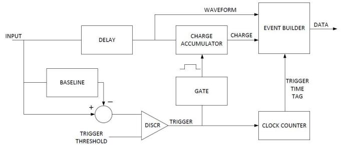
Fig. 6. Schematic representation of the CAEN DPP-CI firmware implementing the charge integration algorithm. (Adapted from [8]).
