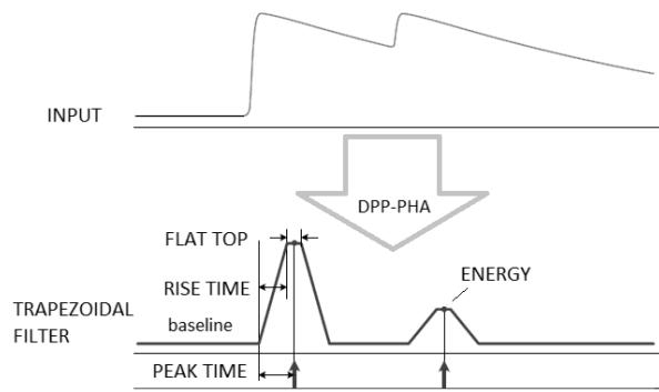
Fig. 8. Operation of the digital trapezoidal filter used in the CAEN DPP-PHA firmware. (Adapted from [11]).
