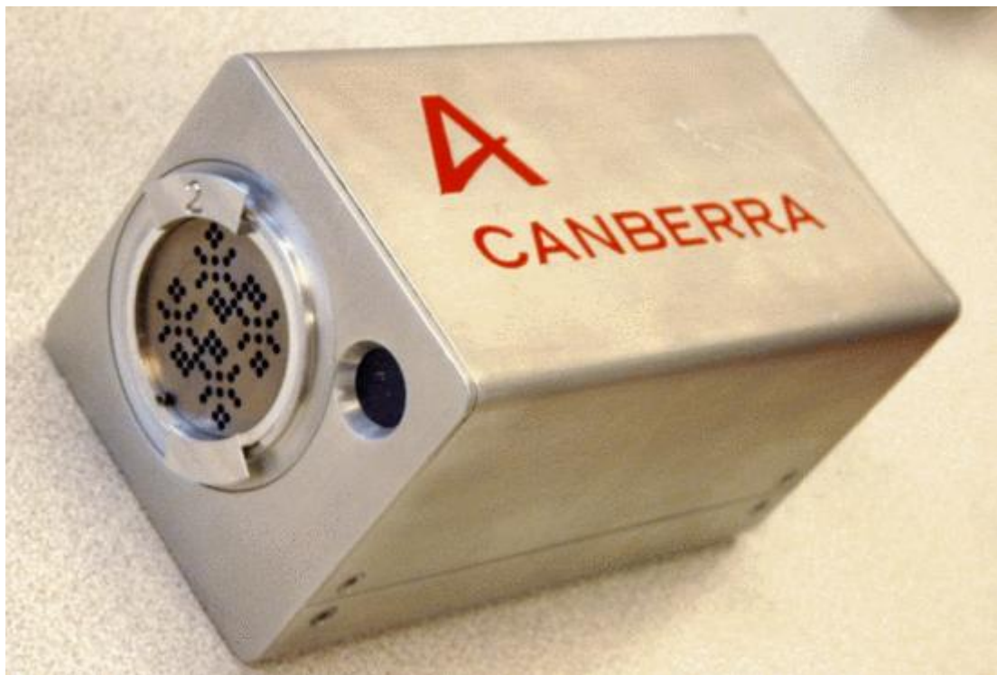
Fig. 1 First industrial prototype of the new generation gamma imager.
