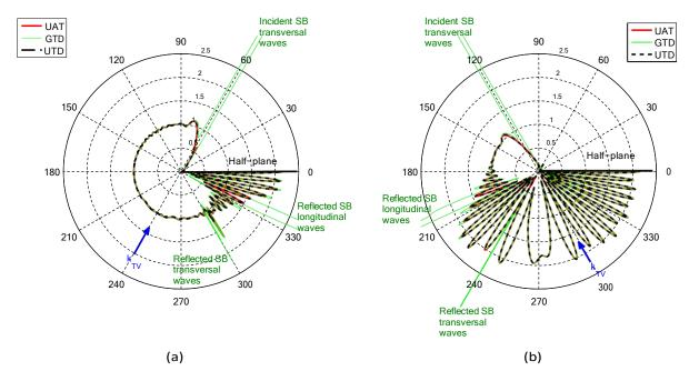
Figure 5: Directivity pattern of the total field predicted by different models (GTD, UAT and UTD) at  $r = 10\lambda$  ( $k_{\beta}L_{\beta} = 20\pi$ ,  $\beta = TV$ ) for  $\Omega_{TV} = 90^{\circ}$  - (a)  $\vartheta_{TV} = 60^{\circ}$  - (b)  $\vartheta_{TV} = 120^{\circ}$ . Each circle represents amplitude of the total field normalized by the incident amplitude.
