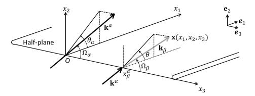
Figure 2: A plane wave of propagation vector  $\mathbf{k}^{\alpha}$  incident on a semi-infinite stress-free crack. Thick black arrow - direction of the incident wave; thick gray arrow - direction of the diffracted wave ( $\mathbf{k}_{\beta}$ ).
