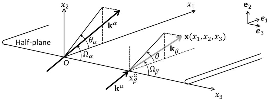
Figure 2: A plane wave of propagation vector  $\mathbf{k}^\alpha$  incident on a semi-infinite stress-free crack. Thick black arrow - direction of the incident wave; thick gray arrow - direction of the diffracted wave ( $\mathbf{k}_\beta$ ).
