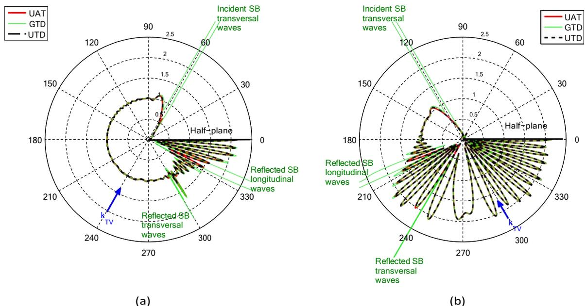
Figure 5: Directivity pattern of the total field predicted by different models (GTD, UAT and UTD) at  $r = 10\lambda$  ( $k_\beta L_\beta = 20\pi$ ,  $\beta = TV$ ) for  $\Omega_{TV} = 90^\circ$  - (a)  $\vartheta_{TV} = 60^\circ$  - (b)  $\vartheta_{TV} = 120^\circ$ . Each circle represents amplitude of the total field normalized by the incident amplitude.
