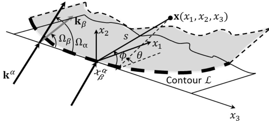
Figure 3: A plane wave of propagation vector  $\mathbf{k}^\alpha$  incident on a stress-free obstacle (in gray) of contour  $\mathcal{L}$ . Thick black arrow - direction of the incident wave; thick gray arrow - direction of the wave  $\mathbf{k}_\beta$  scattered by the half-plane tangent to the crack edge at the flash point  $x_\beta^\alpha$ .
