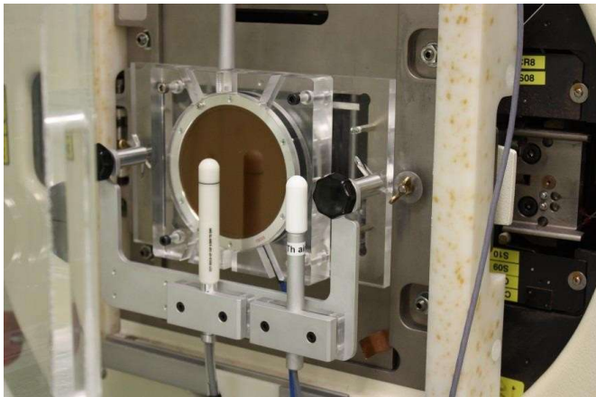
Figure 3. The BIPM monitor chamber support in PMMA, fixed on a shadow tray attached to the LNHB accelerator head. The circular transmission chamber is in the centre. The thimble monitor chamber with build-up cap is positioned directly in front of the transmission chamber. A thermistor in a similar cap is positioned to the right of the chamber and measures the temperature under conditions that simulate those of the thimble chamber. The temperature probe for the transmission chamber is placed vertically at the top of the support. A horizontal metal bar can be positioned between the black knobs providing a geometrical reference plane. The thimble chamber is used for long-term beam monitoring and is removed during the actual measurements.
